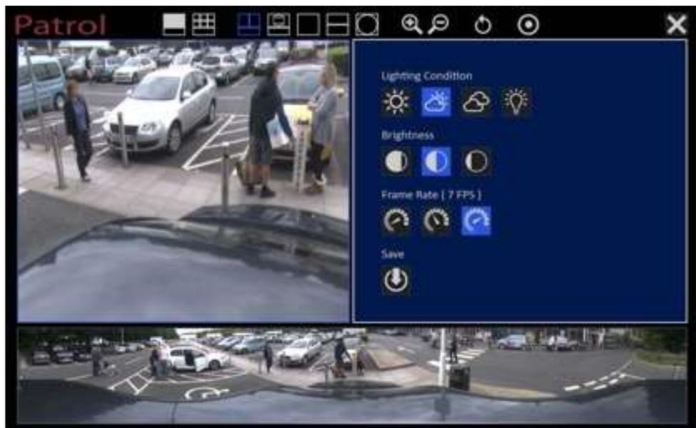
The diagram is a screenshot of the CAMERA applications. This window displays the camera set up tools allowing operators to adjust core settings for exposure, lighting and frame rate. Settings can be saved for ease of operation.
