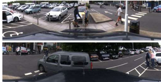
2D split panorama displaying 180° forward and back – or rotated by virtual Pan (vP) value
